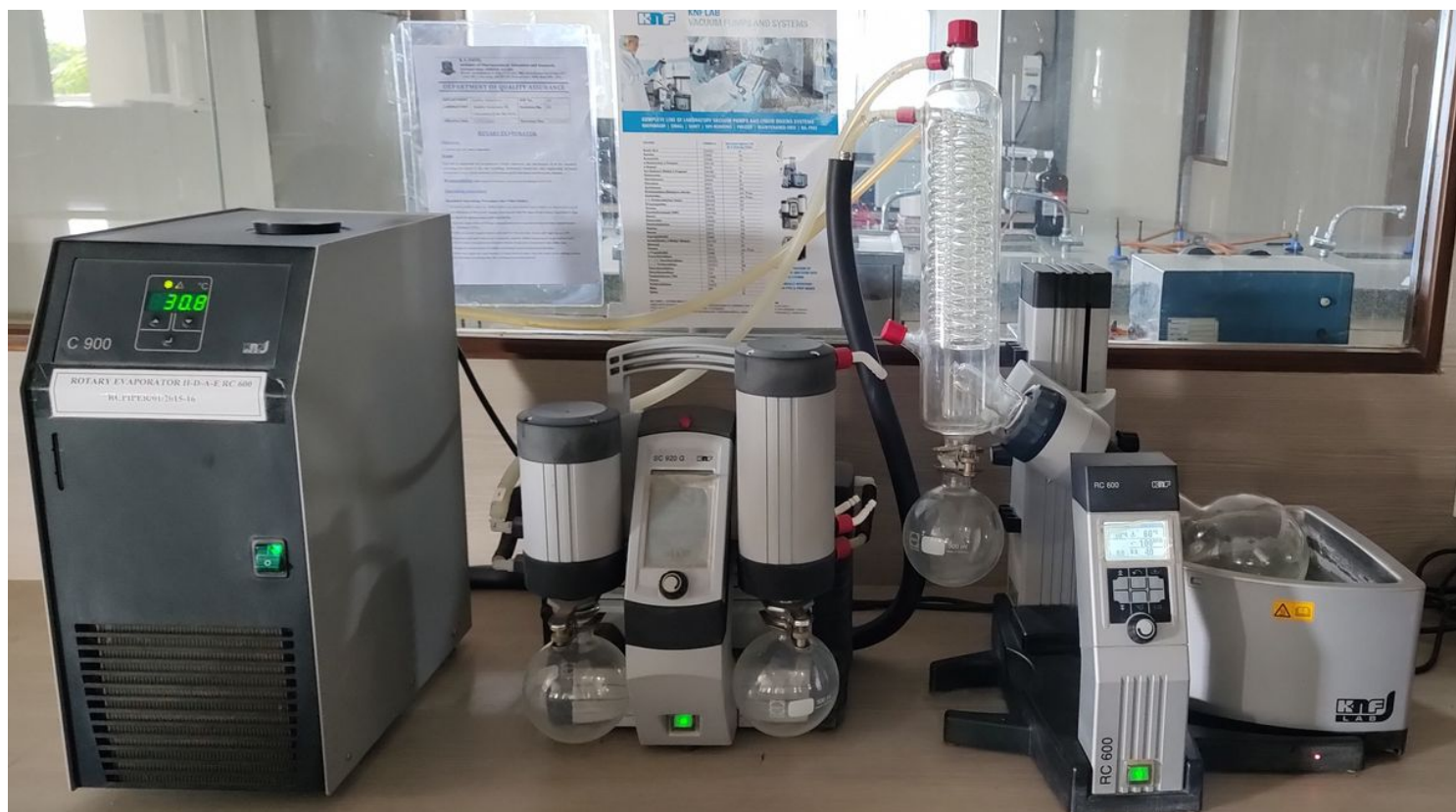
Figure 1 rotary evaporator for preparation of niosomal formulation
