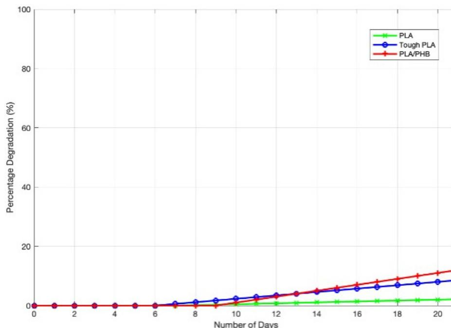
**Figure 6.** Biodegradability test for the fabrication of ureteral stents.
