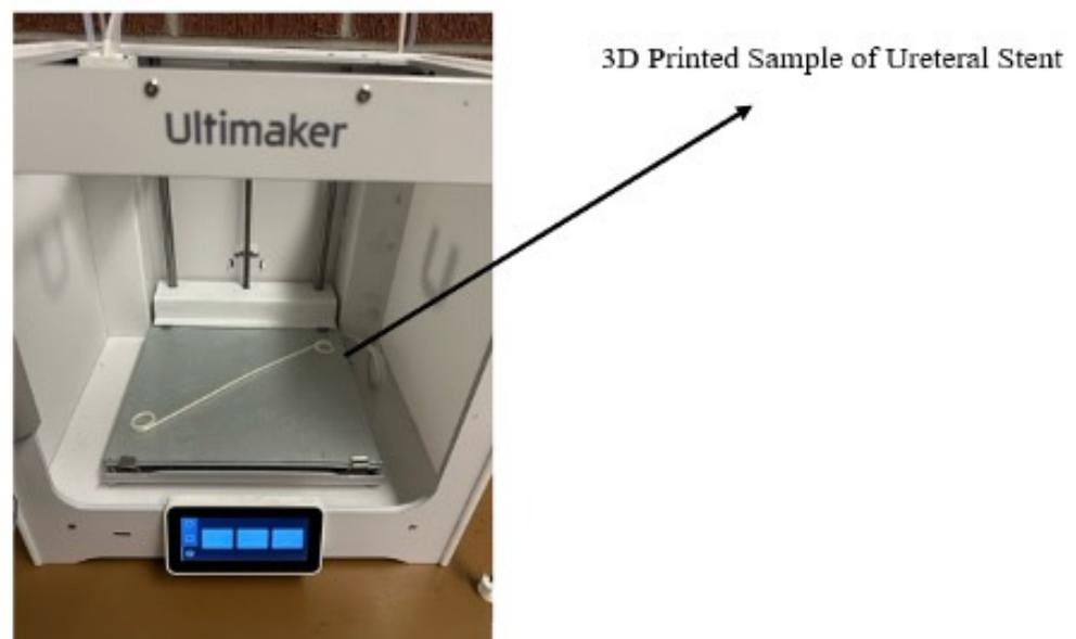
**Figure 2.** Three-Dimensional printing setup used for fabricating the ureteral stent.
