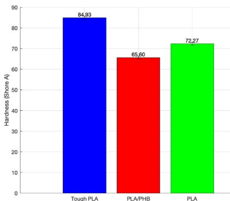
**Figure 8.** Hardness test results for the Tough PLA, PLA/PHB, and PLA stent materials.
