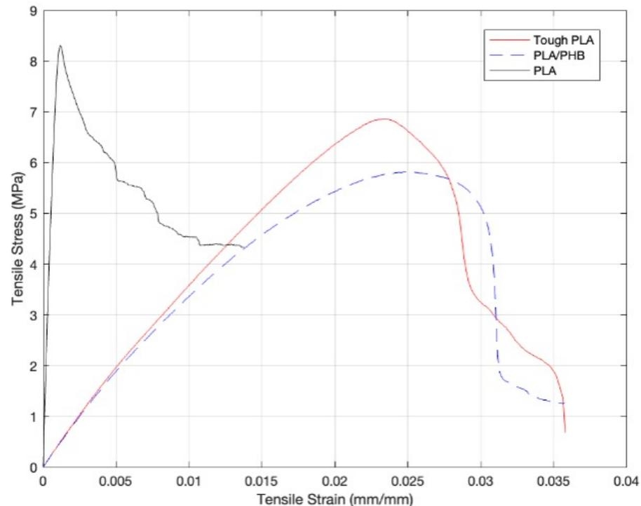
**Figure 7.** Tensile stress vs. Tensile strain plot for the ureteral stent materials.
