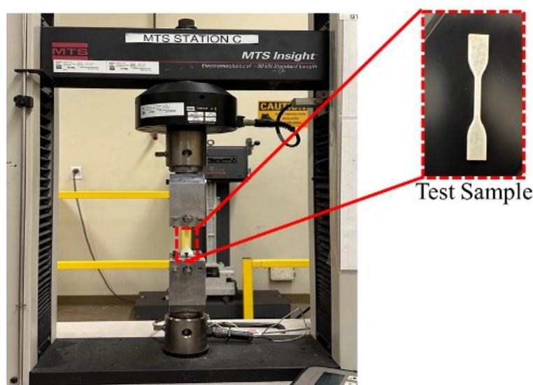
**Figure 3.** Tensile test setup used (inset shows the ASTM 638D-based tensile test sample).
