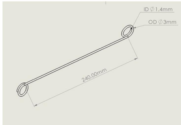
**Figure 1.** CAD of a ureteral stent.
